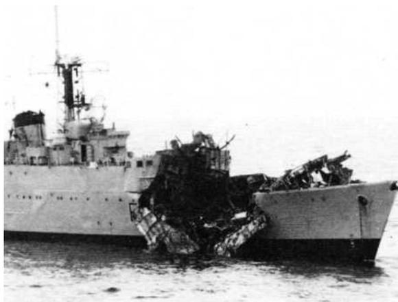
This photo of the old target frigate *Undaunted*, after being struck forward by an Exocet fired on the range by HMS *Norfolk*, proves beyond question that the AM.39 which struck *Sheffield* on 4 May did not, in fact, explode. The damage done by a detonating Exocet warhead is shown here to be so gross that *Sheffield's* loss would have been much quicker, and her casualty list many times longer. (MoD via MARS)
