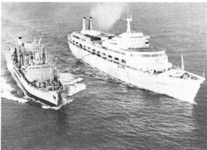
The troopship SS *Canberra* refuels from the RFA *Tidespring* using the abeam transfer method. During a short refit before sailing the liner was fitted with two helicopter landing stations, which can be seen over the forward swimming pool and aft of the bridge, as well as replenishment equipment. (MoD)
