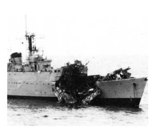
This photo of the old target frigate Undanted, after being struck forard by an Exocet fired on the range by HMS Norfolk, proves beyond question that the AM.39 which struckSheffieldon 4 May did not, in fact, explode. The damage done by a detonating Exocet warhead is shown here to be so gross that Sheffield's loss would have been much quicker, and her casualty list many times longer. (MoD via MARS)
