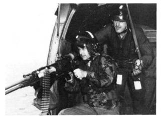
A rather more direct method of hitting the enemy is employed by a Commando Sea King HC.4 of No.846 Sqn operating from HMS *Hernes*—a twin GPMG mount in the door, operated by Sgt. Hannah RM with RN CPO Aircrewman Kelly as loader. Many Commando helicopters were fitted with door guns for selfdefence against ground fire, and to give support to troops. (MoD)
