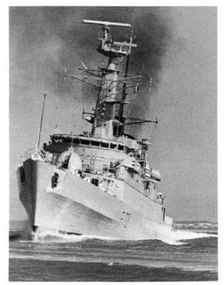
Pre-war shot of HMS *Antelope*, the Amazon class frigate lost on the morning of 24 May after a 5001b bomb, which lodged in the engine room during a raid on the previous day, exploded while being defused and set fire to her fuel. (MoD)
