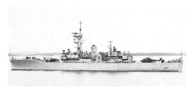
The frigate HMS *Phoebe* following refit and in Falklands grey colour scheme; a number of changes have already been made as a result of combat experience. Note twin 20mm Oerlikon mount on top of the bridge, replacing the MRS 3 director for the forard Sea Cat; this latter was mounted in front of the Exocets, but has also been removed. The boat davits abreast the funnel have been replaced by a Searider inflatable and crane. (C. & S. Taylor)
